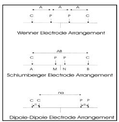
Figure-5: Standard Electrode Geometries.Source: Abstracted from ASTM D6431-99 (2005)
