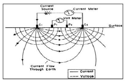
Note: C1 and C2, P1 and P2 refer to the current and voltage/potential electrodes respectively.
