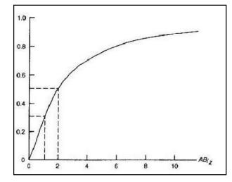
**Figure-6:** Fraction of current penetrating below a depth Z for a current electrode separation AB Proportion of current flowing below depth Z (Source: Telford, Second Edition)
