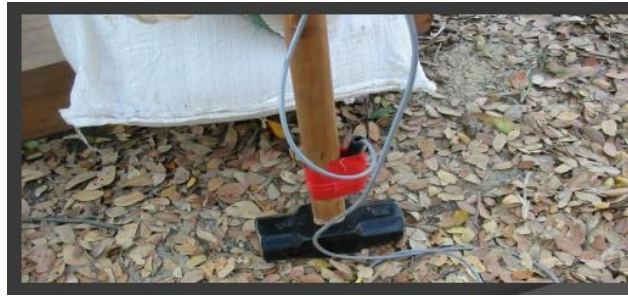
Figure 3.6 To attach the trigger to a hammer.
