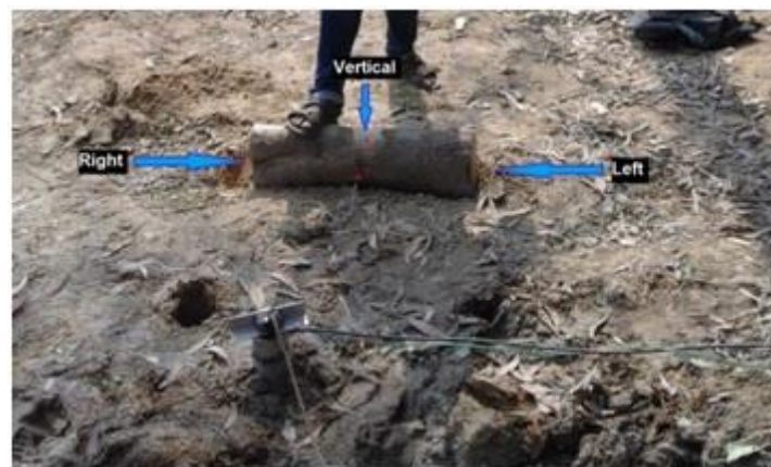
Figure 3.10 Hit the wooden plank in 3 directions which are on the left, right and vertical directions.
