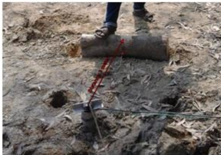
Figure 3.5 To set the wooden plank and sand bag 3.0 meters from a borehole
