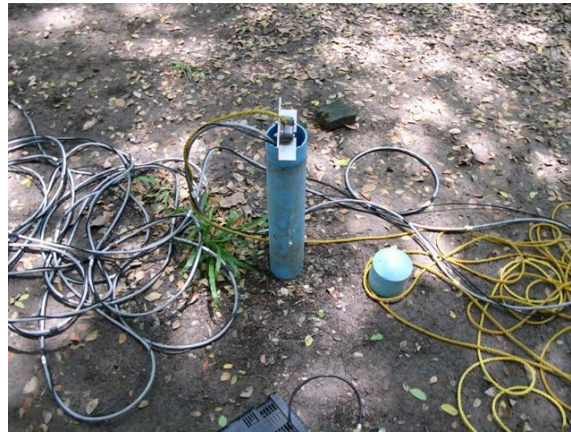
Figure 3.9 Make sure that the air bag at the geophone works. Then, put the geophone into the borehole and fix the safety rope with the holder
