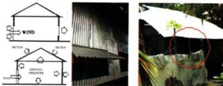
Figure 9 Corresponding opening on the leeward side may reduce the internal wind pressure
