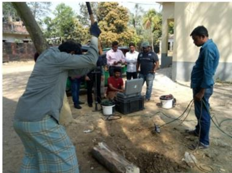
Figure 3.1 Field Data Acquisition by PS logger
