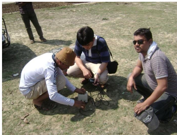
Figure 3.5 Field data acquisition of Single microtremor
